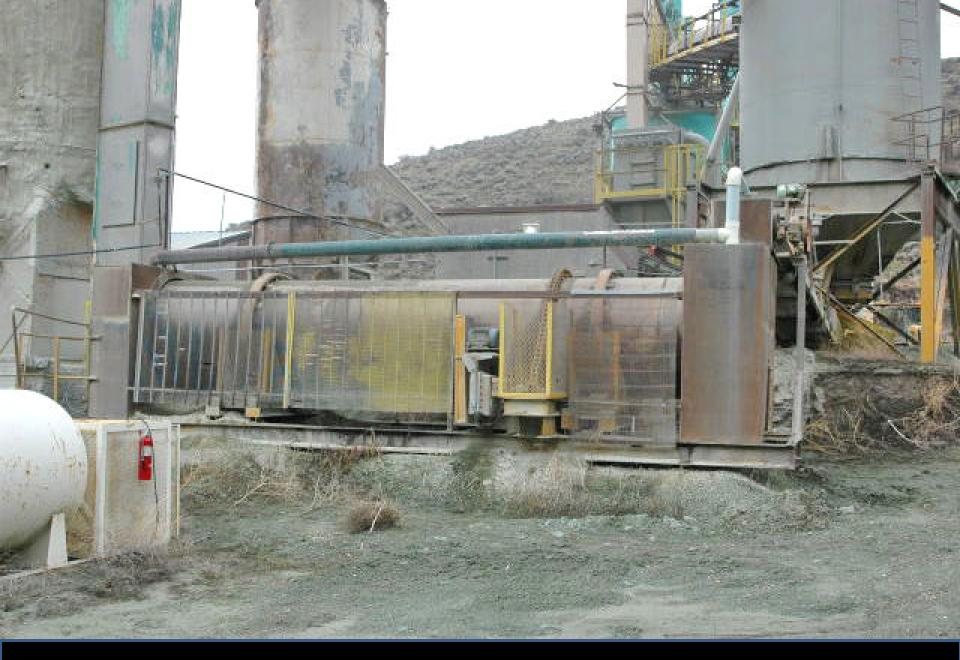
Dryer feed bin on right for Raymond mill and liners 1 and 2 for granular products.
