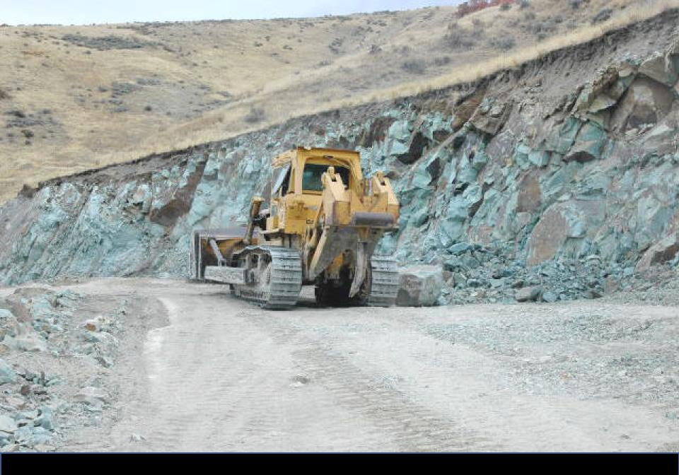
Face of zeolite in front of D8K with ripper.
