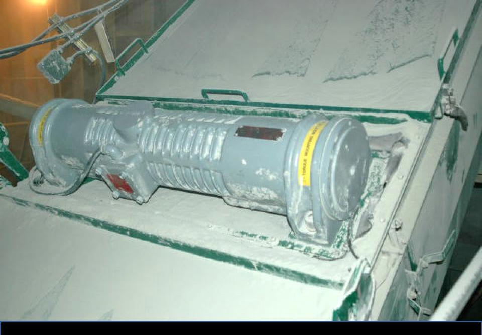
Derrick 3600rpm high frequency screen for line one.
