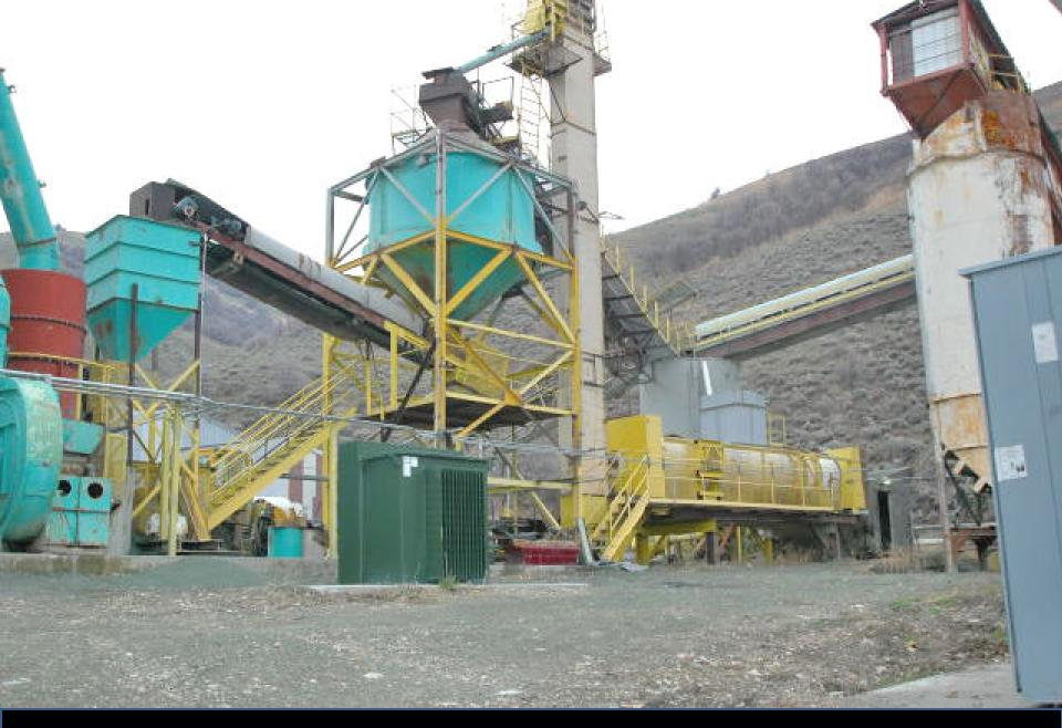
Raymond mill feed -- dryer or dryer bypass; bucket elevator; feed bin; conveyor; surge bin to feeder on mill.
