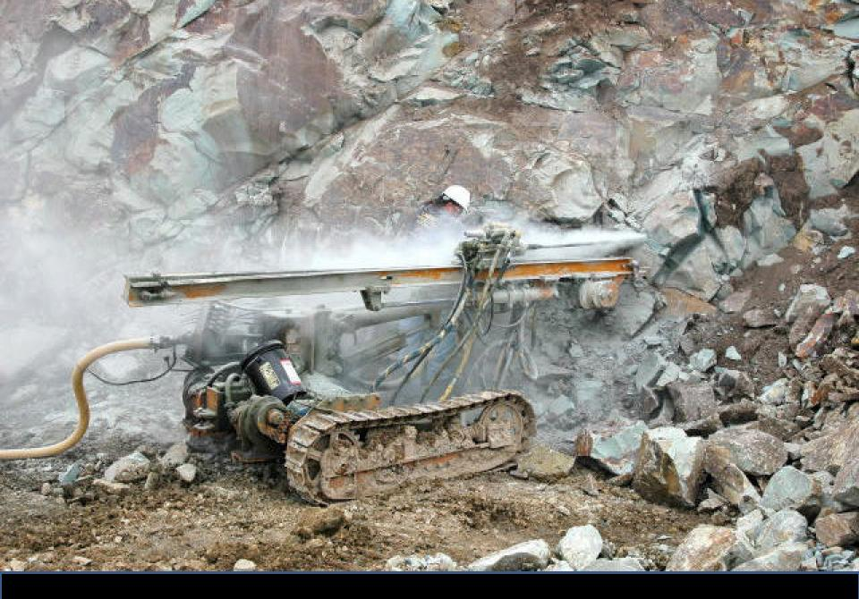
Blowing blast hole air track.
